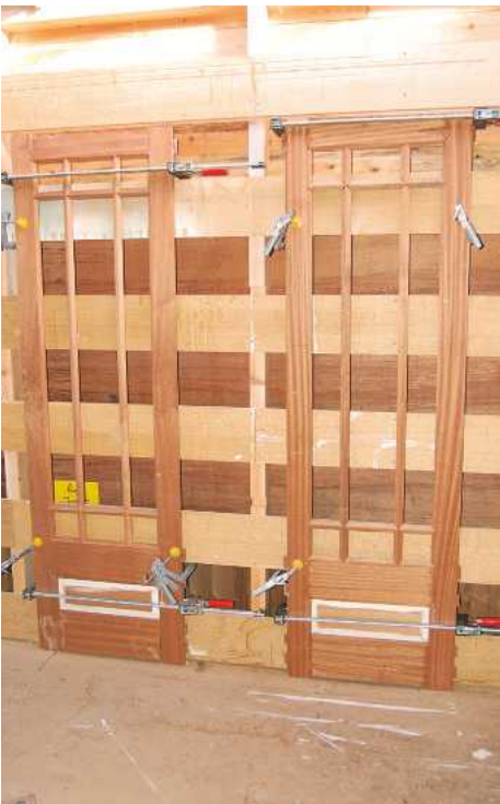
▲ Pic.21 The doors could then be clamped and glued up
